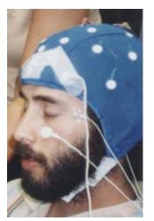
Figure 1: Electrode Cap with Quick Inserts
