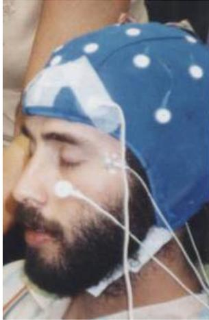
Figure 1: Electrode Cap with Quick Inserts
